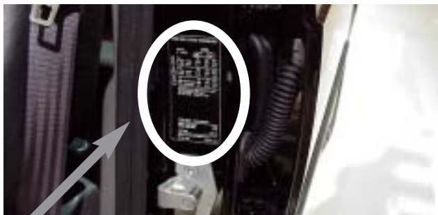
= SAAB 9-5 = VIN PLATE LOCATION
