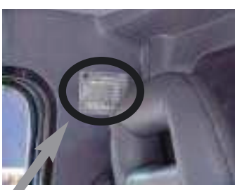
NISSAN CABSTAR VIN PLATE LOCATION
