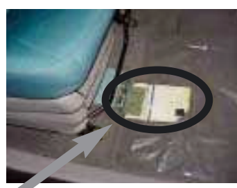
NISSAN ALMERA TINO VIN PLATE LOCATION
